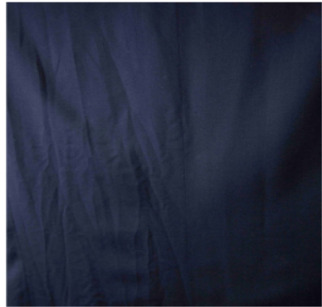
Running marks (creases in the warp direction) are caused by permanent setting during the dyeing process.
