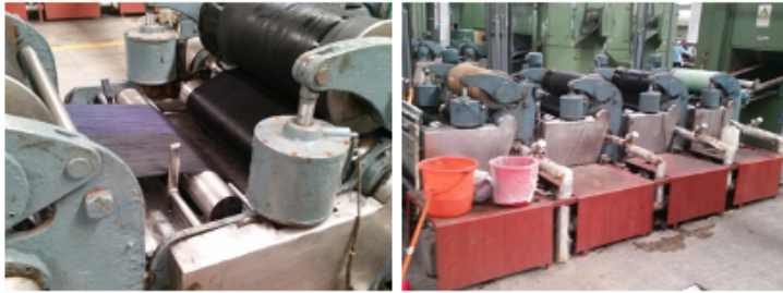
Backwash showing bowls and squeeze rollers
