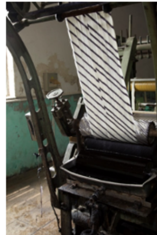
Worsted top can be dyed (left) or printed (above) before further processing occurs
