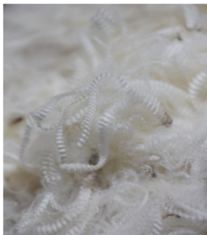
Crimp is observable as 'waves' in the raw fibre.
