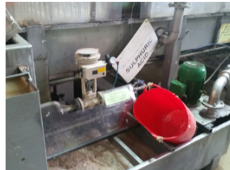
Additions tank on a carbonising line showing addition of sulphuric acid
