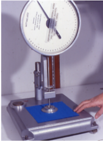
Fabric thickness meter for assessing pressing
