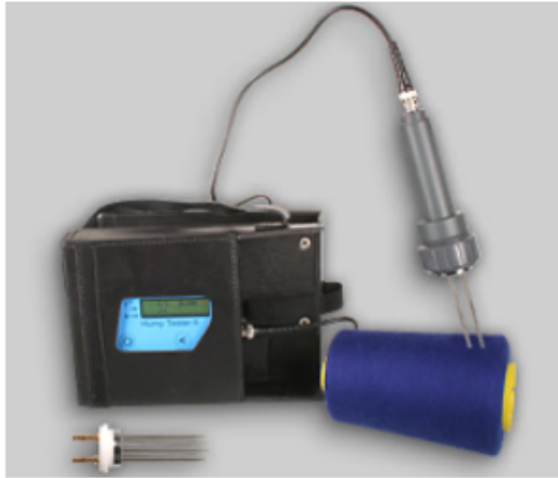
Meter for measuring fabric moisture content
