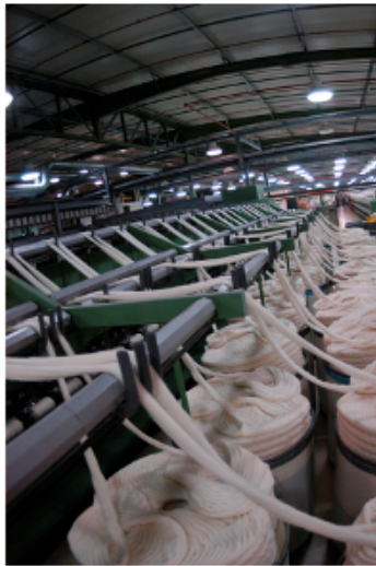
The creel (at left) showing the creel rollers (at right)
