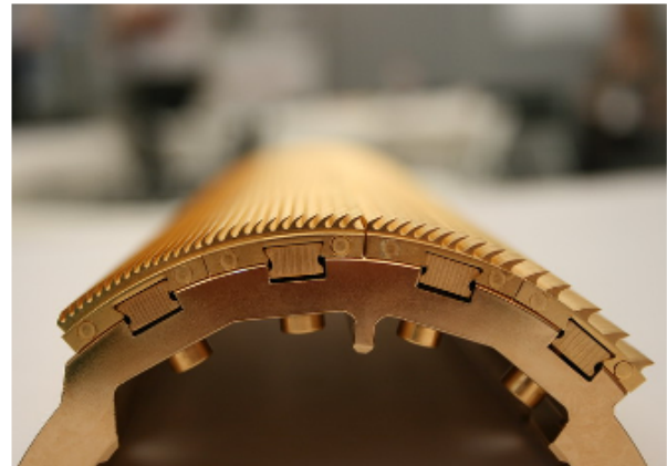
Pins on circular comb (finer pins on the left segment)
