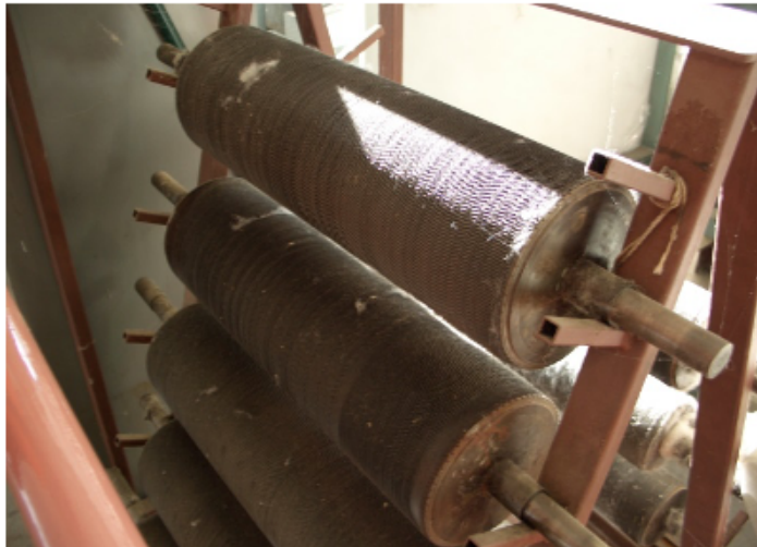
Rollers from a narrow-width card removed for cleaning
