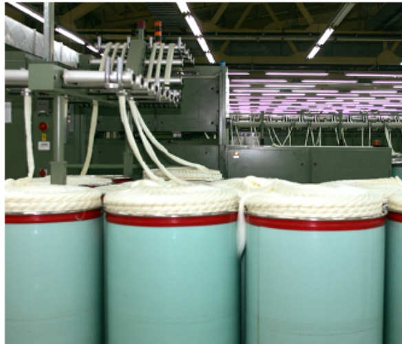
Input slivers being fed into gill box
