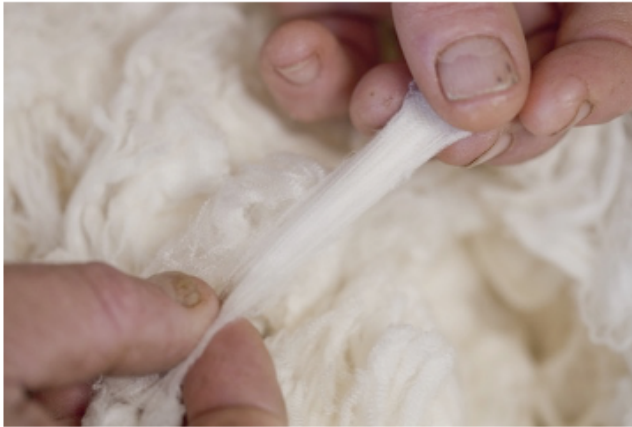
Staple length is measured in raw wool and recorded on the AWTa certificate
