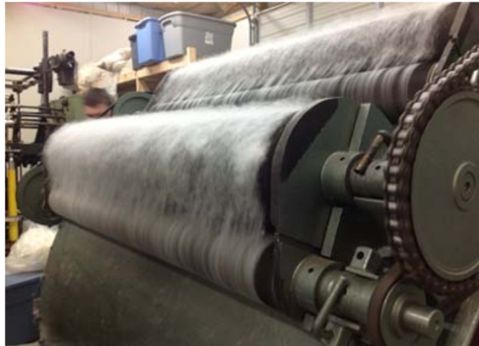
Commercial carding equipment (worker and stripper rollers)
