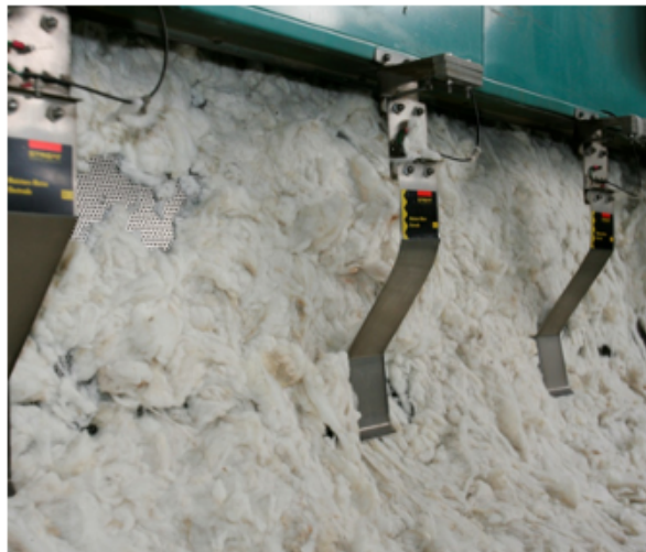
Moisture meters on exit to dryer following scouring
