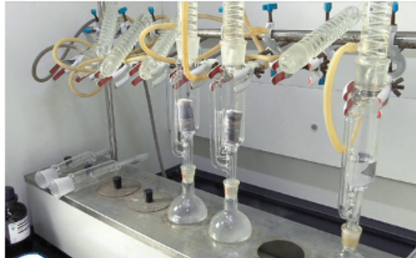
Soxhlet apparatus to extract residual contaminants
