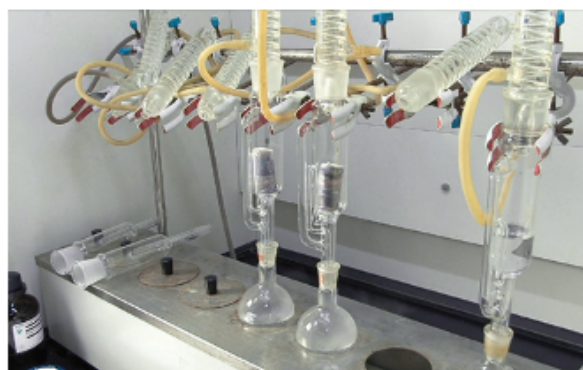
Soxhlet apparatus to extract residual contaminants
